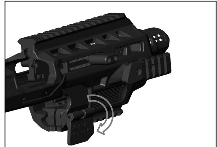
Slide pistol into rail adapter, verify that both sides fit into the receiving profile in the Kidon™.
