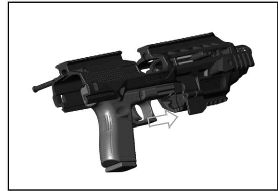
Slide and Click Rear Locking Assembly into place and push Takedown pin back into the body.
